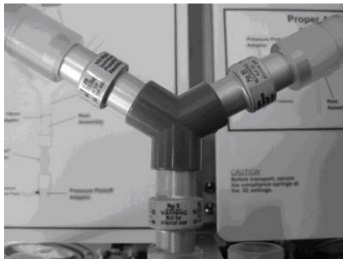
Fig. 4. Adjustable resistive elements modeling the upper airways and bronchial resistance.
