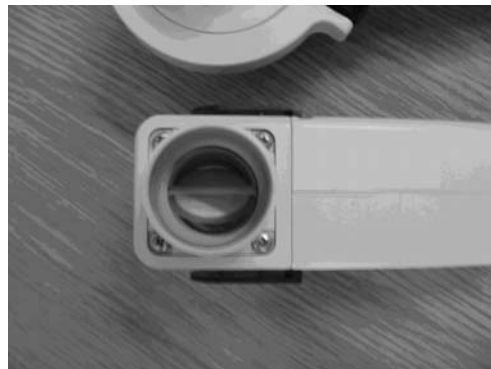
Fig. 6. Medical purpose pressure sensor with embedded shutter.
